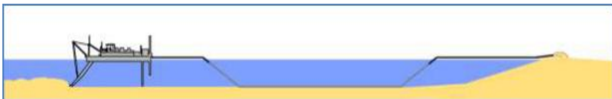
Figure 10.5 CSD Discharging Onshore through Submerged Pipe
