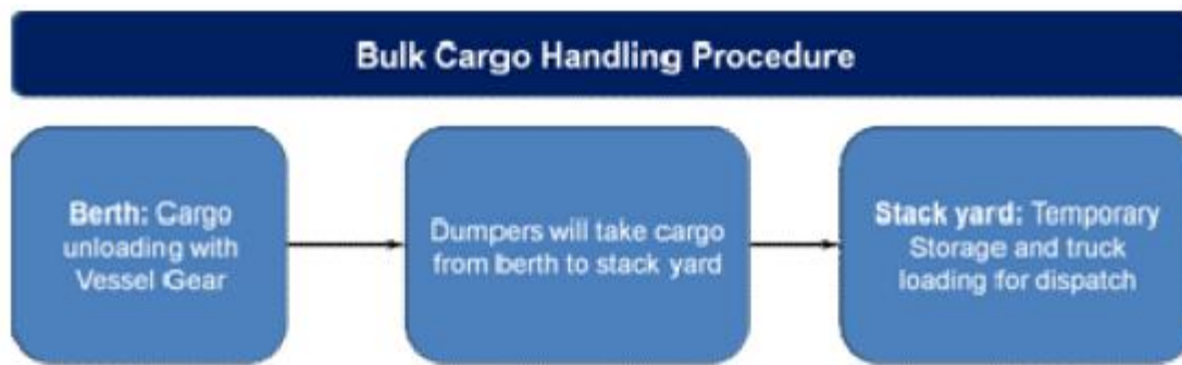
Figure 11.13 Flow Diagram for Multipurpose Cargo Handling System
