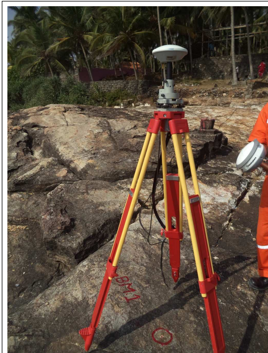
Figure 15 – RTK System fixed at BM-1
