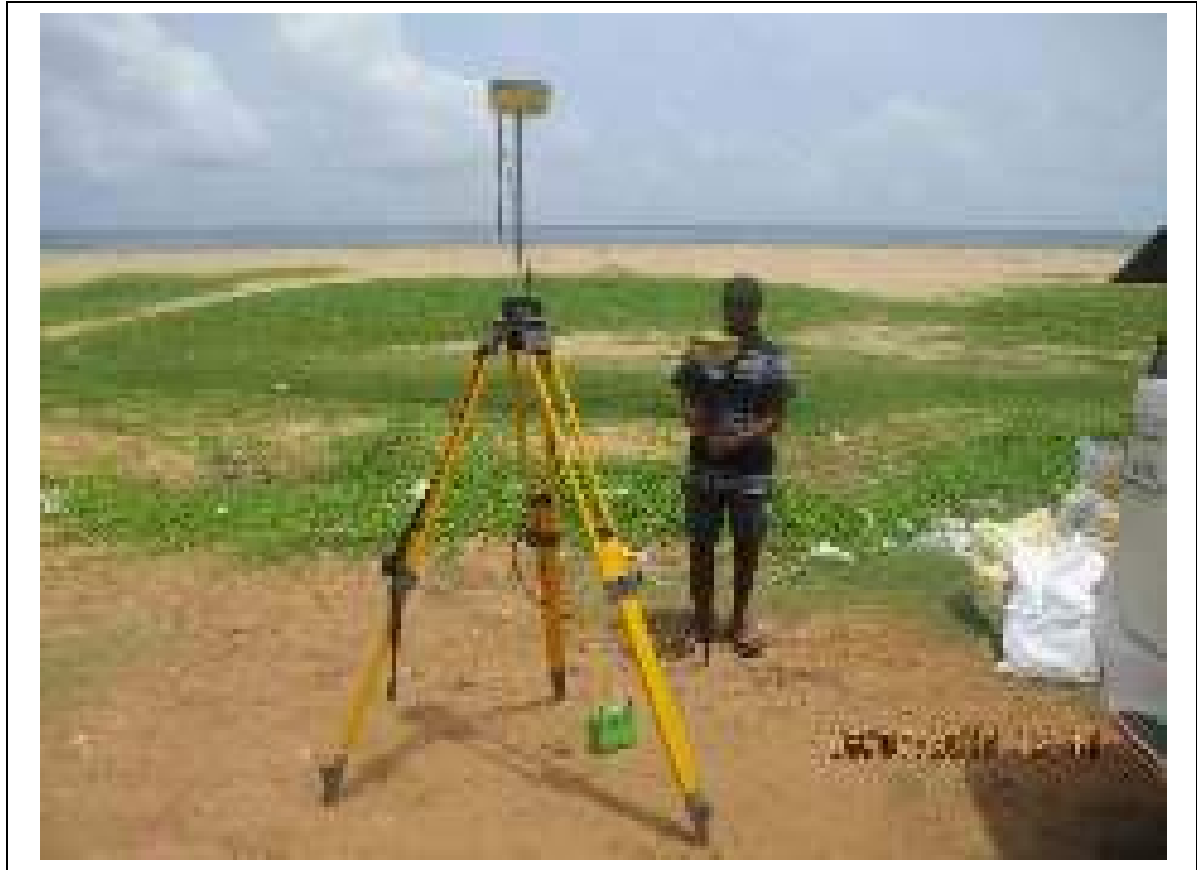
Figure 5-5: RTK System with base station and rover
