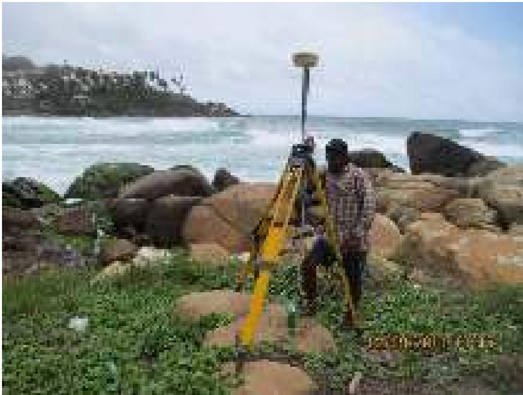
Figure 5-5: RTK System with base station and rover
