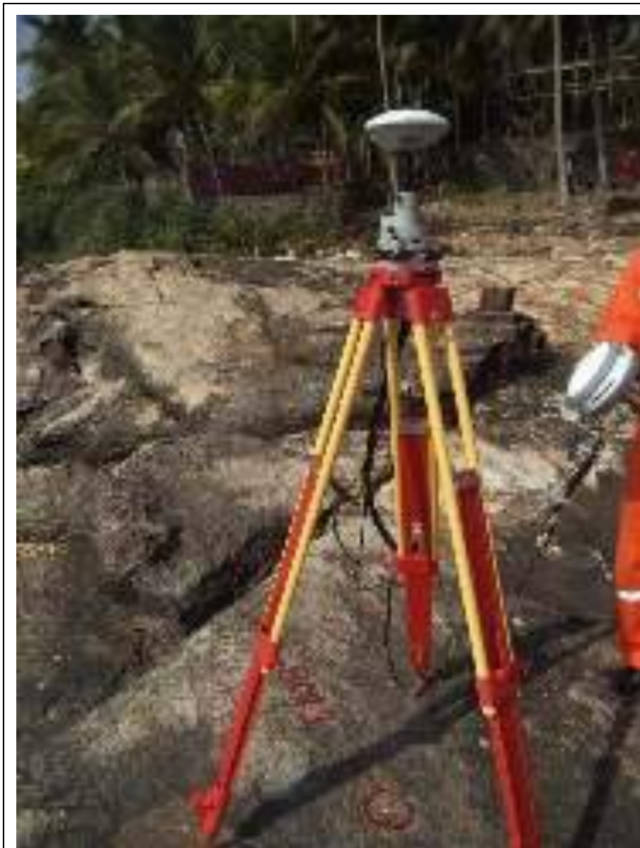
Figure 13 – RTK System fixed at BM-1
