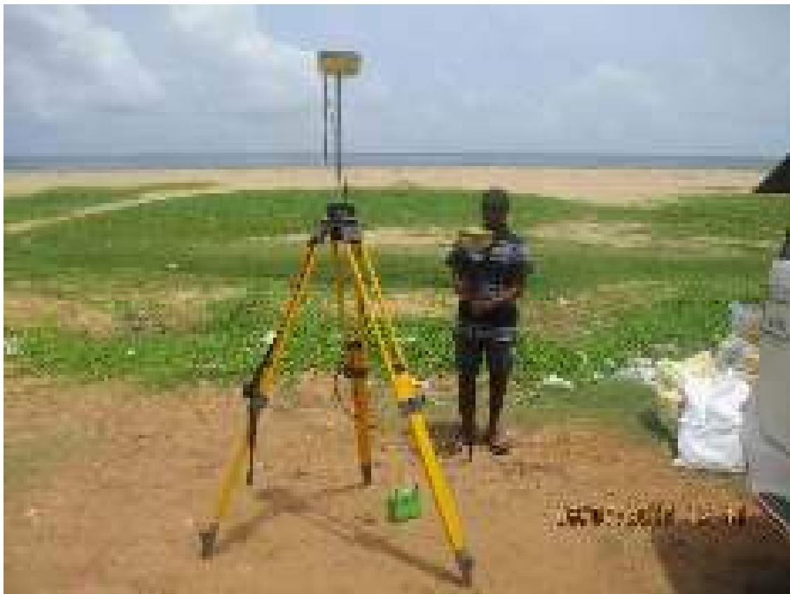
Figure 5-5: RTK System with base station and rover
