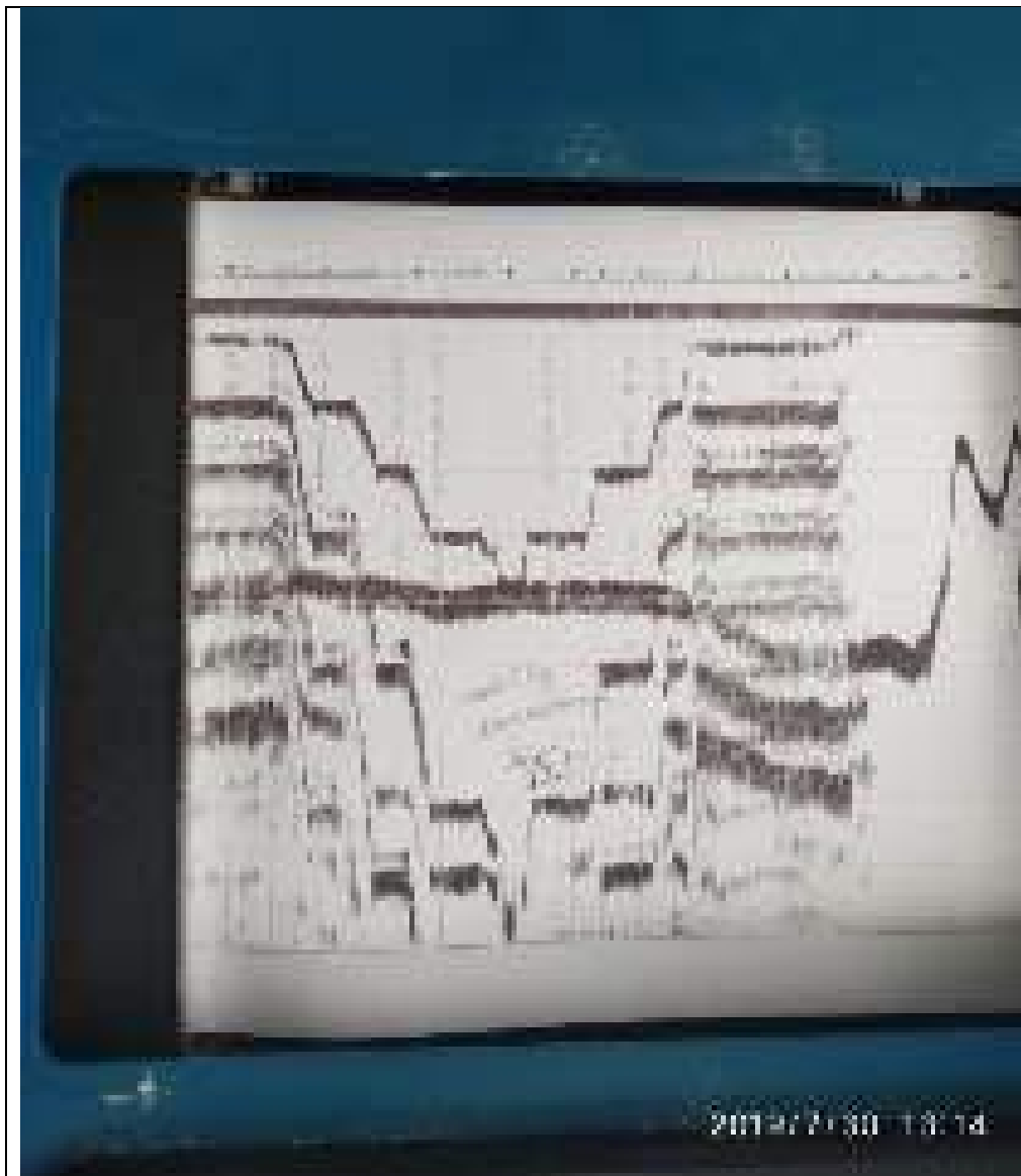
Figure 5-6: Bar check carried out on Syqwest Bathy 500 MF single beam echo sounder
