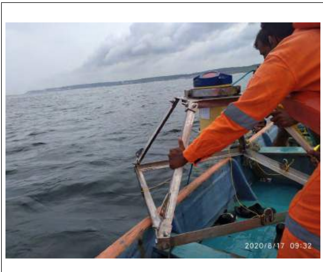
Figure 5-3: ADCP deployment at Vizhinjam by diver
