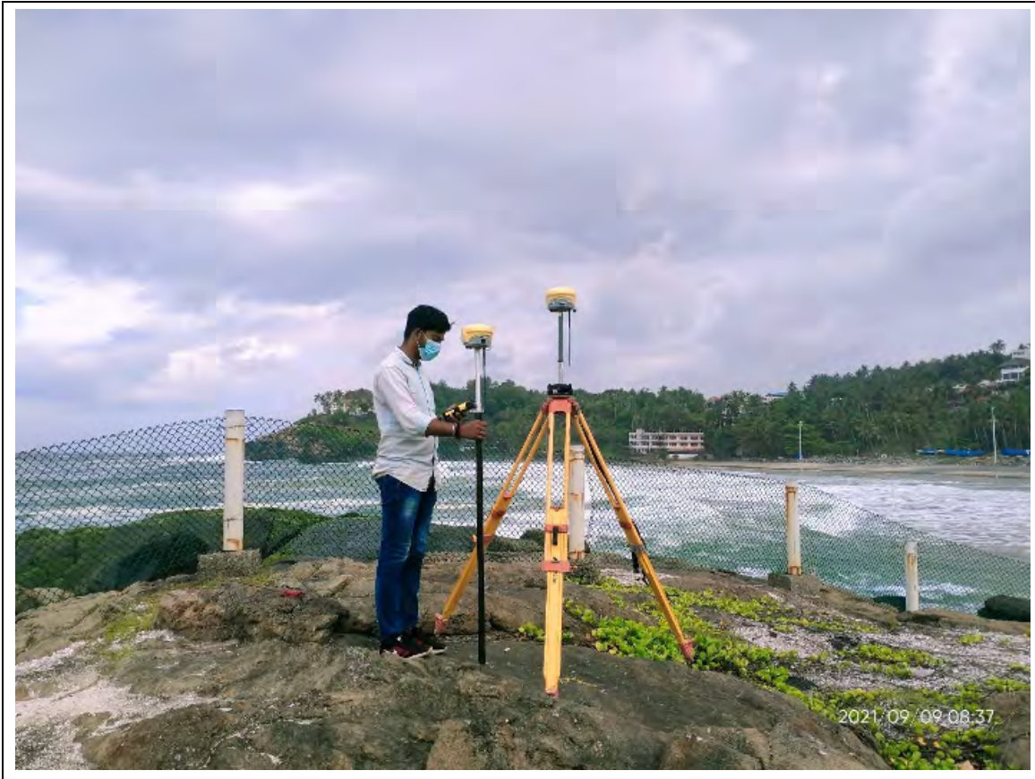
Figure 5-6: RTK System with base station and rover
