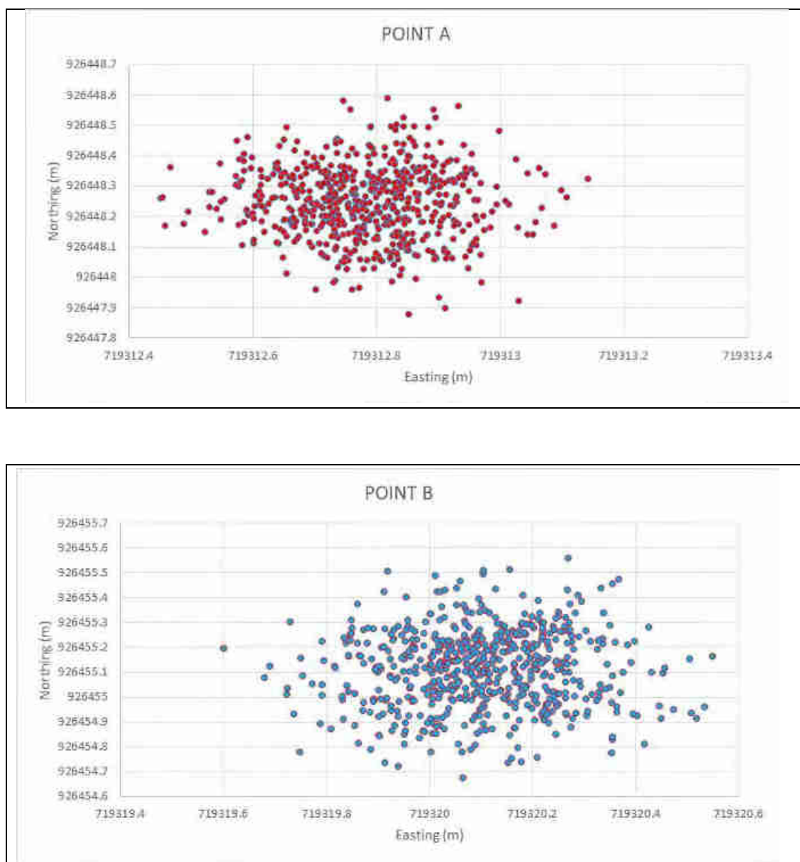
Figure 5-7: Scatter Plot of DGPS calibration on board M.F.B. Bethel
