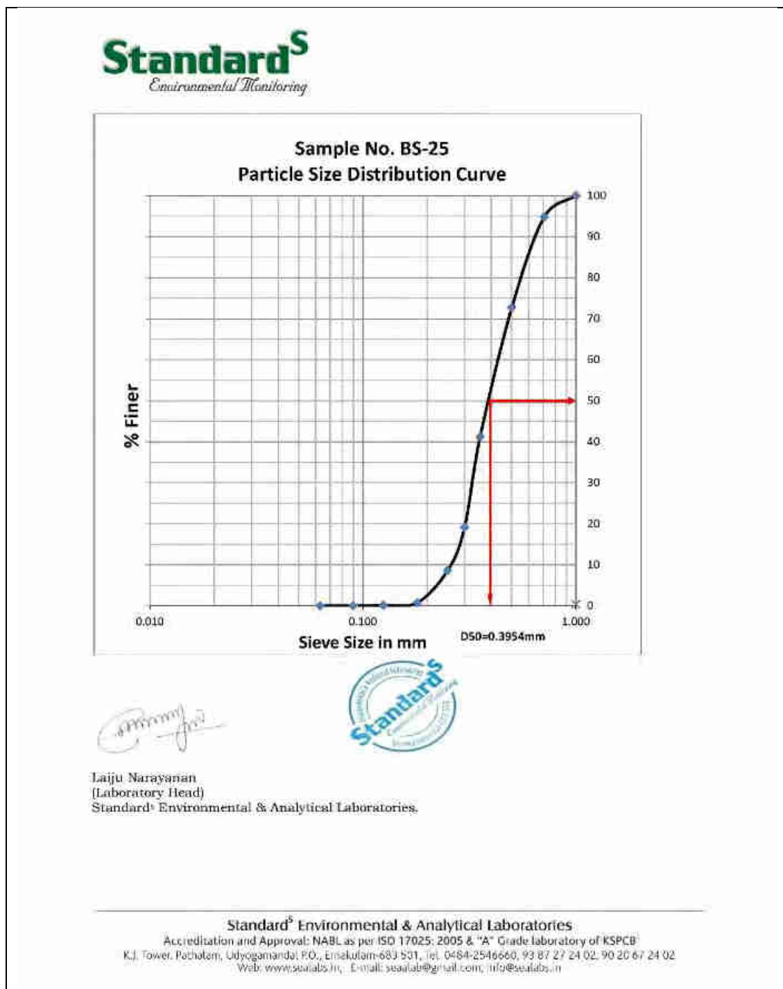
Figure 6-28: Grain size distribution curve for BS-25 (Monsoon)
