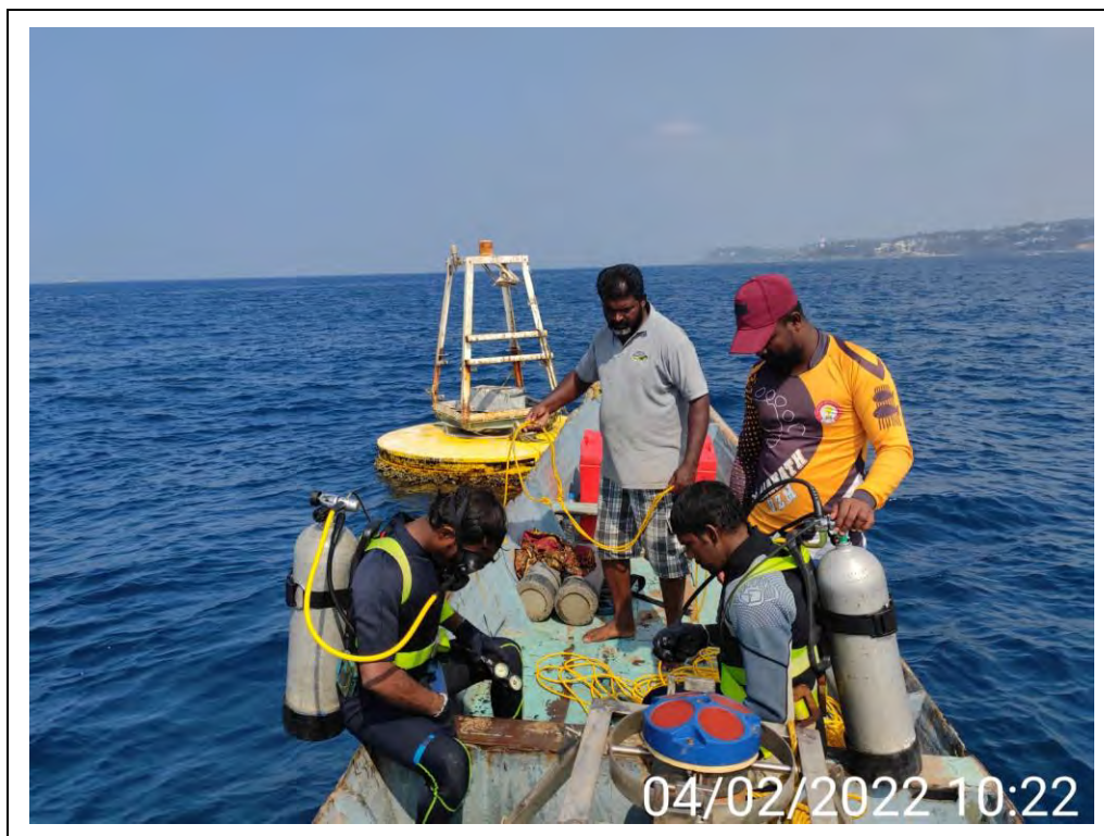
Figure 5-3: ADCP deployment at Vizhinjam
