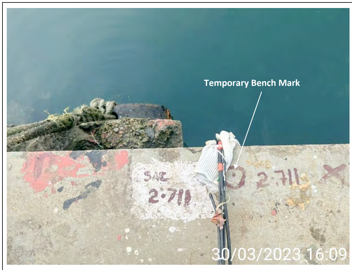
Figure 6-1: Location of TBM
