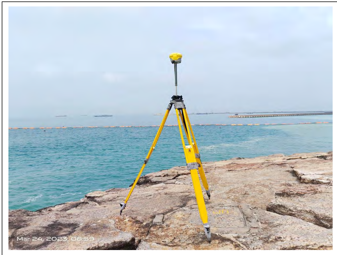
Figure 5-7: RTK System with base station and rover
