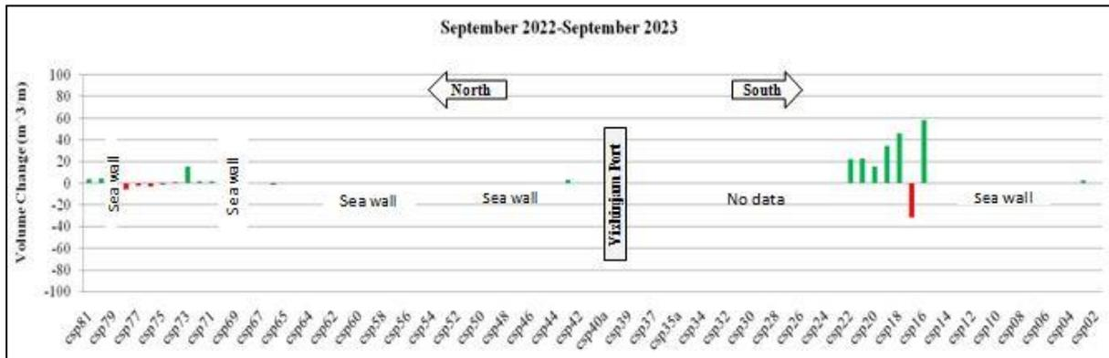
**Figure 4.25 Beach Volume Change comparison between September 2022 and September 2023 in  $m^3/m$  (onshore)**
