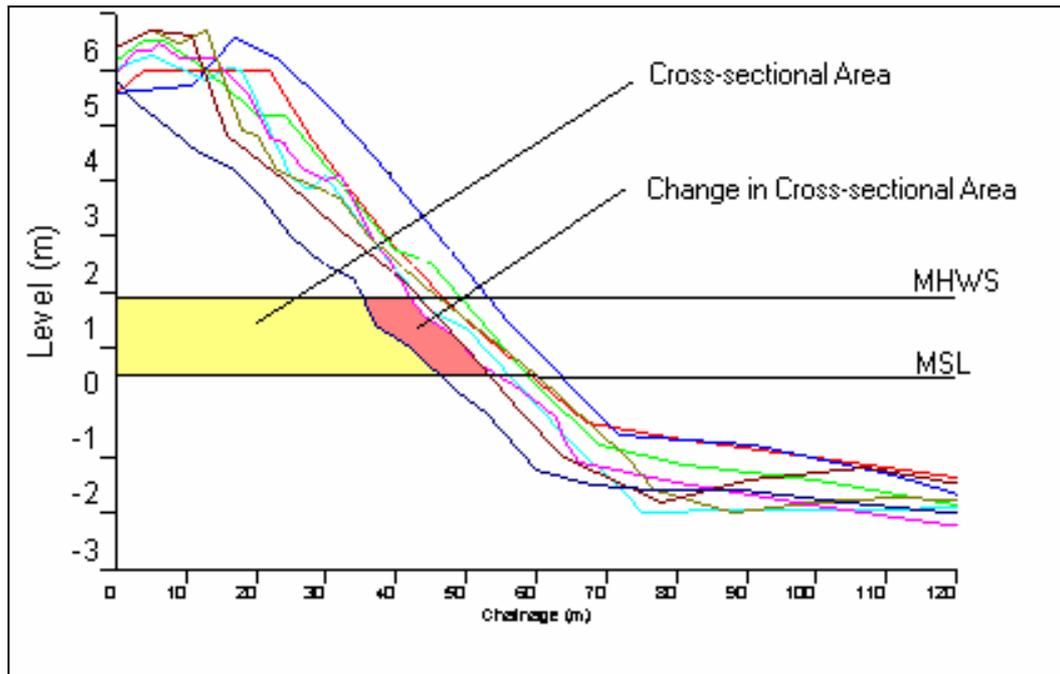
Figure 3.6 Profile Analysis by Level
