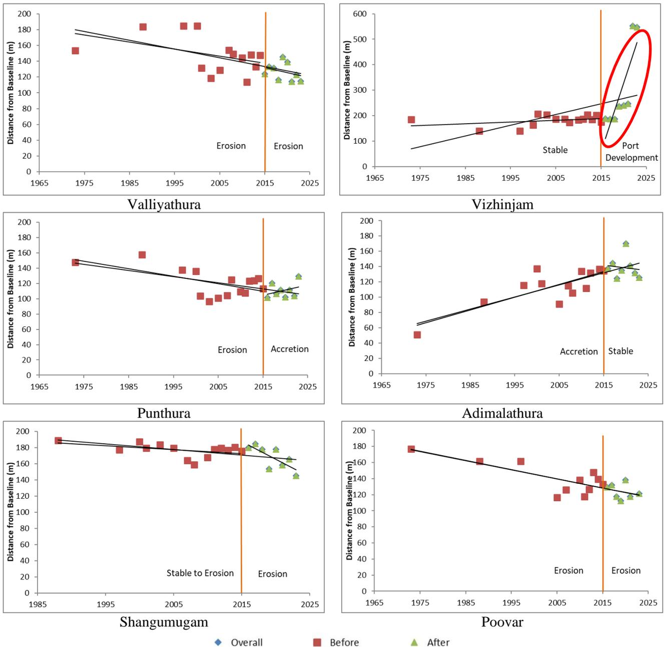
**Figure 5.3** Trend analysis of shoreline change distance from baseline from 1973 to 2022 and trends before and after 2015.
