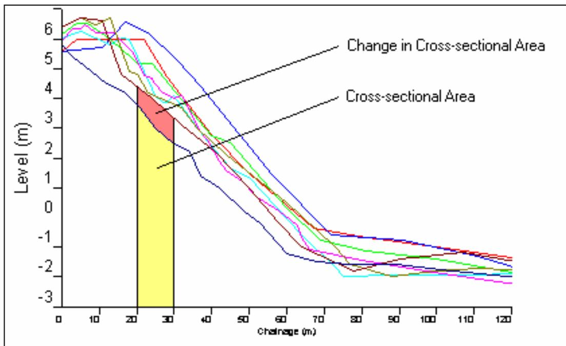
Figure 3.7 Profile Analysis by Chainage
