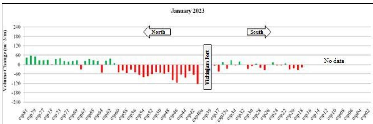
Figure 4.11 Monthly Beach Volume Changes in January 2023 in m<sup>3</sup>/m (offshore)
