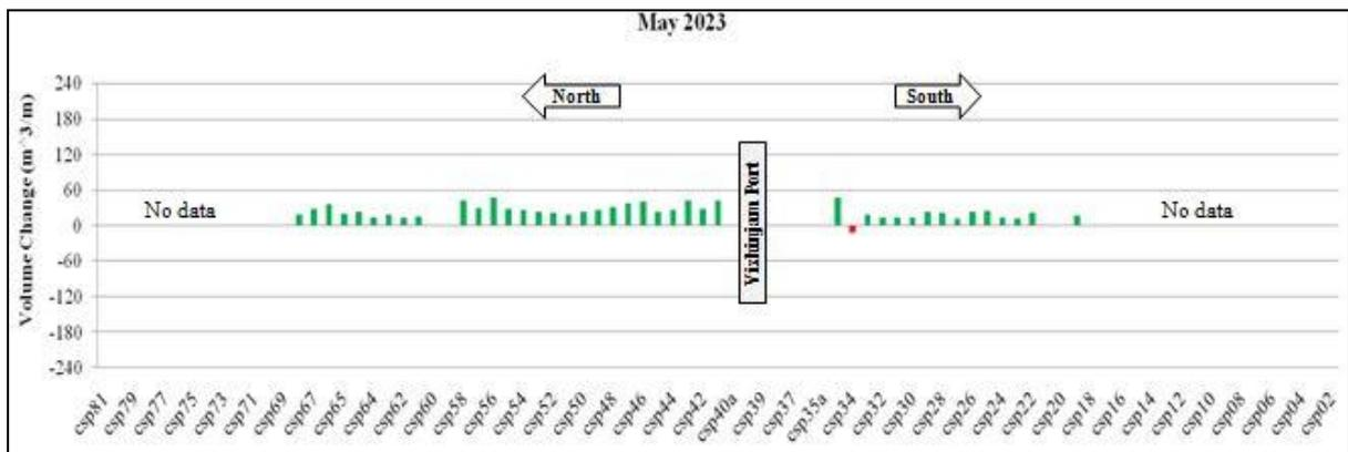
Figure 4.15 Monthly Beach Volume Changes in May 2023 in m<sup>3</sup>/m (offshore)
