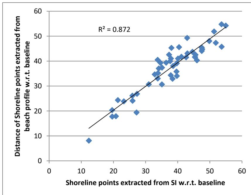
**Figure 5.2 Correlation of shoreline extracted from satellite image and beach profiles.**
