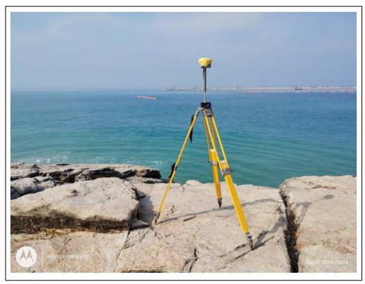
Figure 5-4: RTK System (base station)
