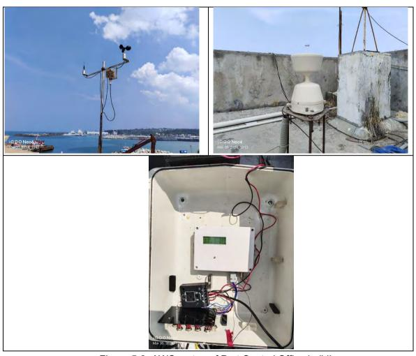
Figure 5-3: AWS on top of Port Control Office building
