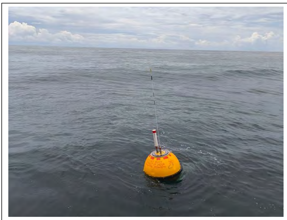
Figure 5-2: WRB deployed at site
